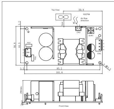
NOTE: Unit: mm SVR1:Output adjustable resistor TOL: ±1.00
