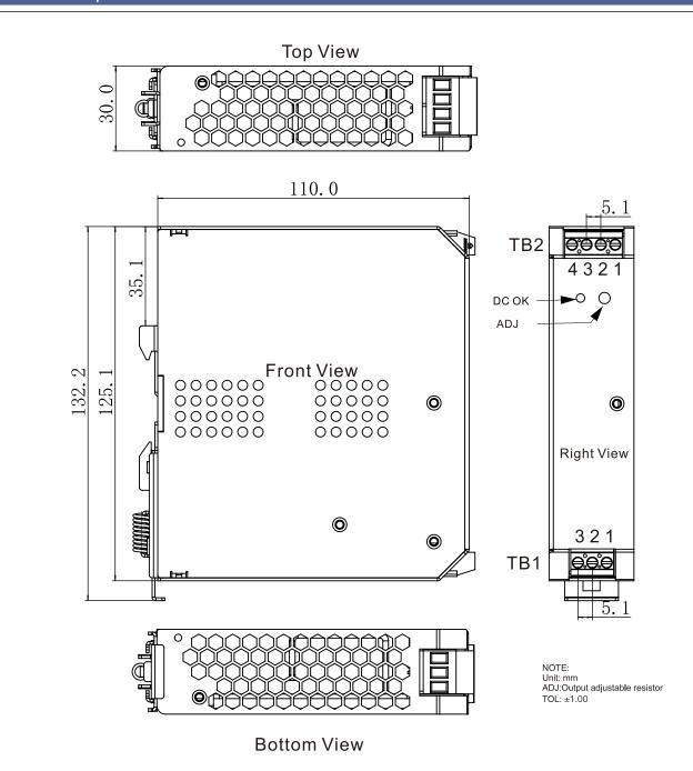
ADMISSIBLE DIN-RAIL:TS35/7.5 OR TS35/15 Terminal Pin No. Assignment
